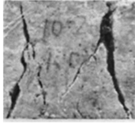
Figure 9: The failure mode under uniaxial compression for concrete sample
