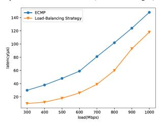
Figure 5: Network latency comparison between ECMP and our load balancing strategy
