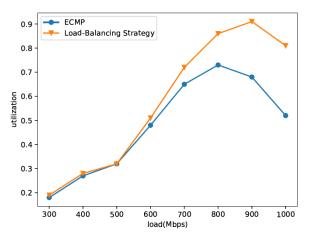
Figure 6: Utilization performance comparison between ECMP and our load balancing strategy
