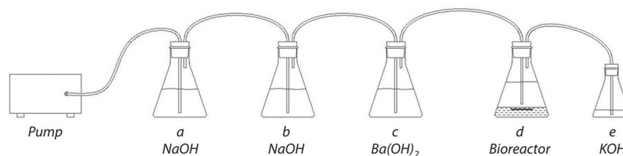
Figure 2 Device for the biodegradation test in marine environment.
