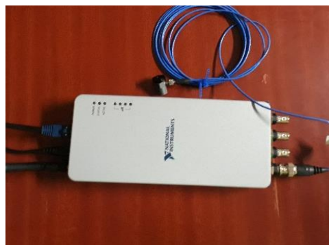
Figure 4: Data acquisition hardware with CDAQ chassis NI9191
