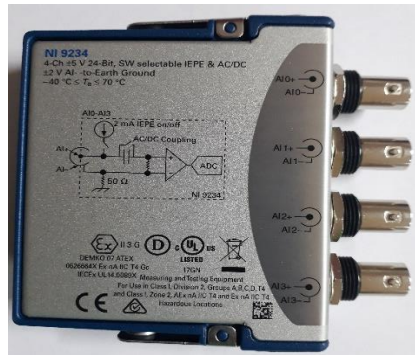
Figure 2: Data acquisition hardware-NI9234-4 channel DAQ
