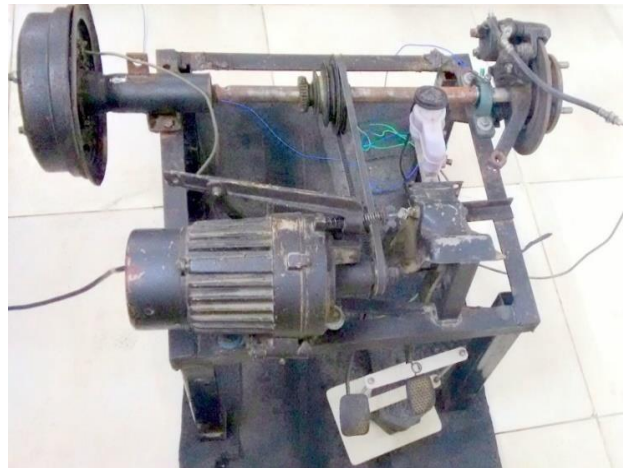
Figure 1: Experimental Setup-Hydraulic Brake system
