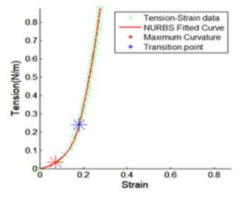
Figure 1. ATAA tension strain curve
