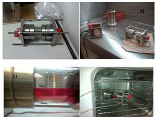
FIGURE 5. A. Bioreactor. B. Bioreactor connected to the peristaltic pump with culture medium (80 ml). C. Bioreactor with culture medium and PLLA scaffold. D. Bioreactor installed within the CO 2 incubator.
