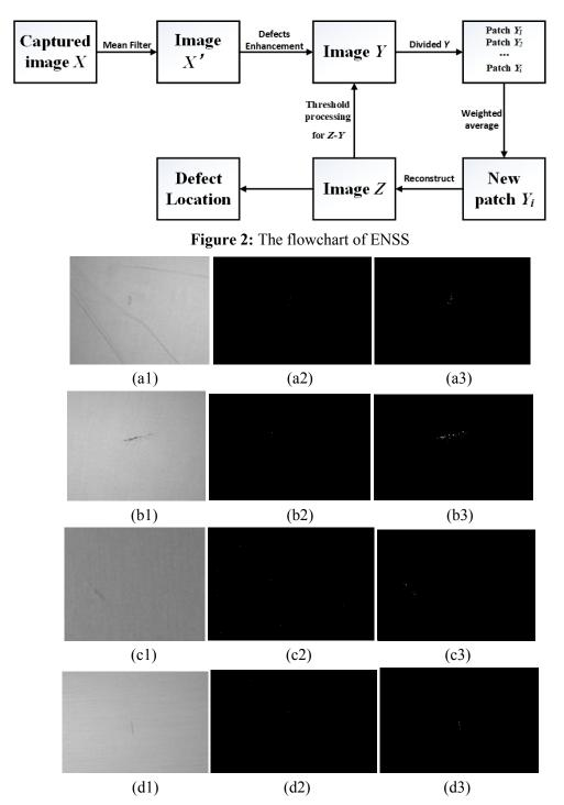
**Figure 3:** Detection results of two methods. (a1)-(d1) are the original images. (a2)-(d2) are the results of Buades et al. [Buades, Coll and Morel (2005)]. Images. (a3)-(d3) are the results ENSS algorithm
