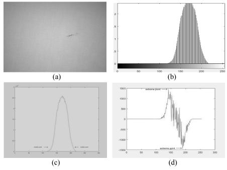
**Figure 1:** Components distribution sample of fabric image (a) A defect image (b) Gray histogram and distribution (c) The envelope curve of gray histogram (d) The first order gradient of gray density function
