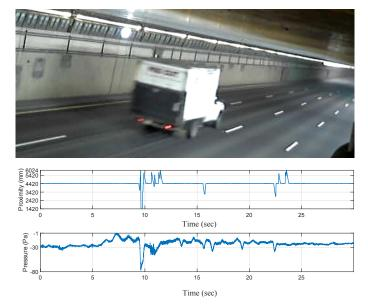
Figure A3. Passage of small box truck.
