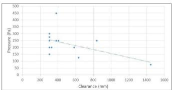
Figure 2. Variation of magnitude of negative pressure with clearance.
