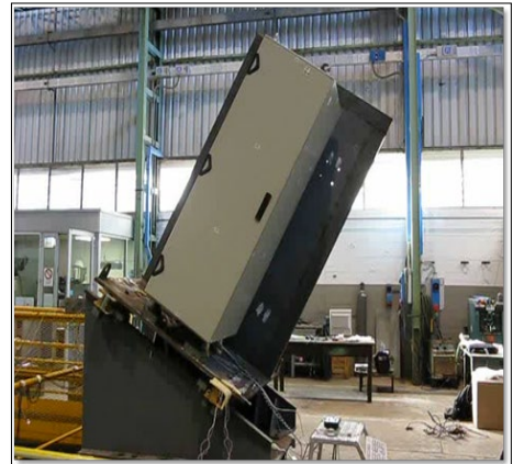
Figure 8. MWSM test setup with Rubber Isolators.
