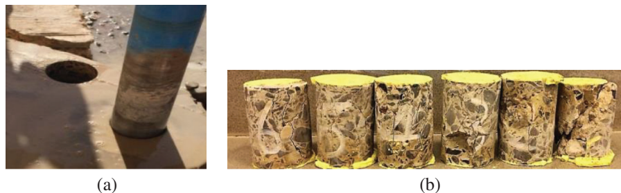
Figure 1: (a) Concrete core sample drilling and (b) samples after testing
