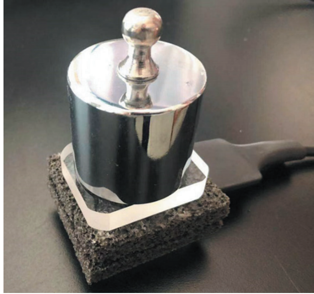
Figure 1: Picture of sensor for transient hot line method
