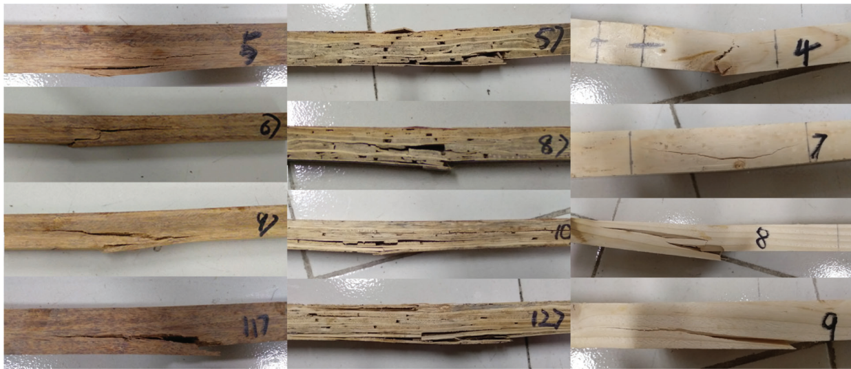
Figure 3: The failure modes of tested specimen (from left to right: bamboo scrimber, bamboo plywood and SPF dimension lumber)
