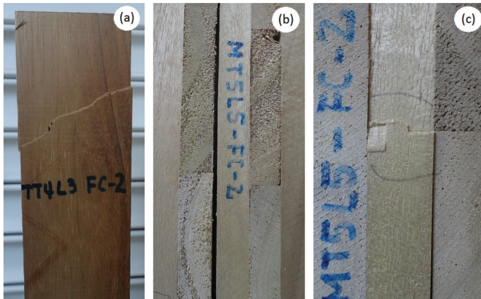
Figure 5: Failures in compression parallel to the grain test: shearing (a), splitting (b) and crushing (c) for the 3- and 5-layer CLT panels of the two species
