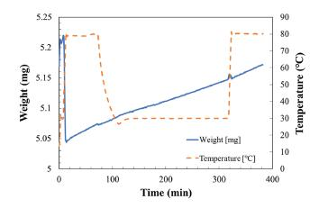
Figure 5: Temperature and weight change in TG at reaction temperature 30°C and relative humidity of 19.3%
