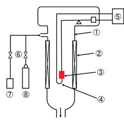
**Figure 1:** Experimental setup for thermogravimetric measurement method Note: ① Reactor; ② Heater; ③ Sample; ④ Thermocouple; ⑤ PC; ⑥ Value; ⑦ Vapor injector; ⑧ N<sub>2</sub> tank
