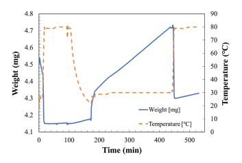
Figure 4: Temperature and weight change in TG at reaction temperature of 30°C and relative humidity of 32.0%
