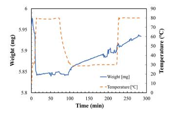
Figure 6: Temperature and weight change in TG at reaction temperature 30°C and relative humidity of 10.2%
