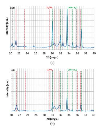
**Figure 3:** The XRD analysis of samples: (a) Raw material before hydration reaction, (b) Material after 15 times of hydration/dehydration reactions
