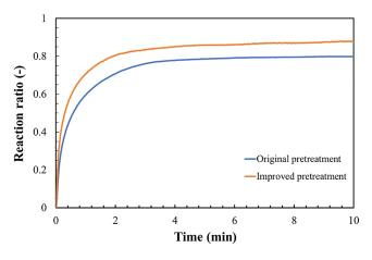
Figure 8: Effect of reducing carbonation (Temperature 47°C, steam pressure 9 kPa, particle size 32–40 µm)
