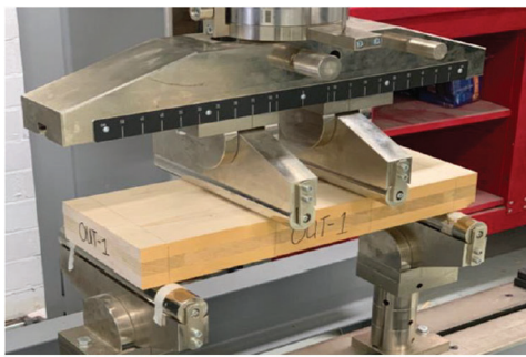
Figure 7: Test set up for short span bending test to determine shear properties
