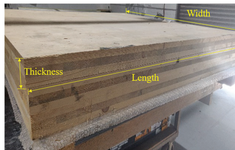
Figure 1: CLT samples produced from Norway spruce
