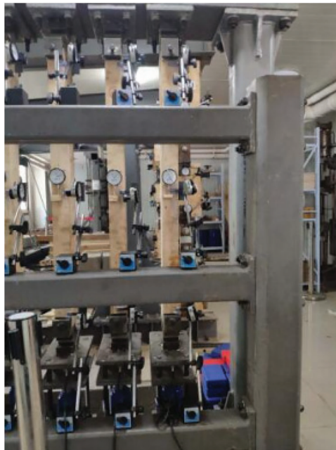
Figure 4: Arrangement of dial indicators
