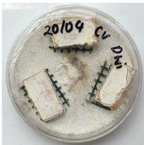
Figure 11: Aspect of wood samples after exposure to Trametes versicolor
