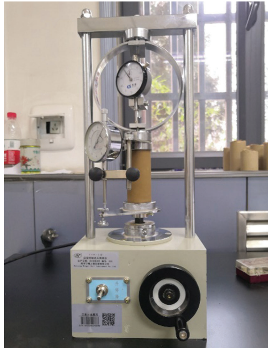
Figure 6: Unconfined compression testing machine with specimen installed
