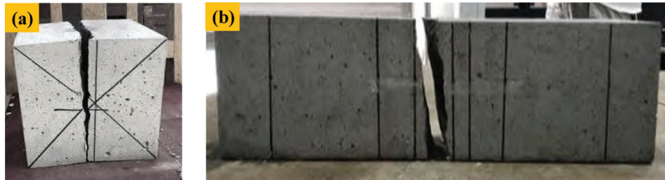
Figure 9: Typical failure mode of tensile and flexural test. (a) Splitting tensile strength; (b) Flexural strength
