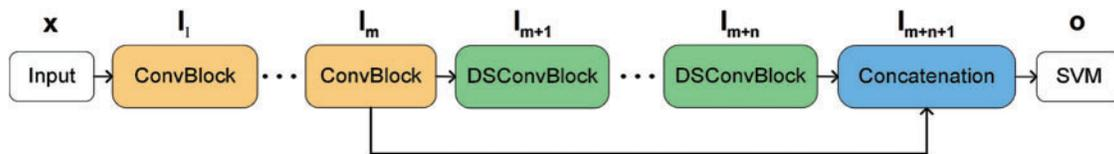
**Figure 1:** A lightweight framework of cross-connected convolution kernel mapping support vector machines
