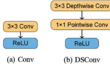
**Figure 2:** Standard convolution and depthwise separable convolution
