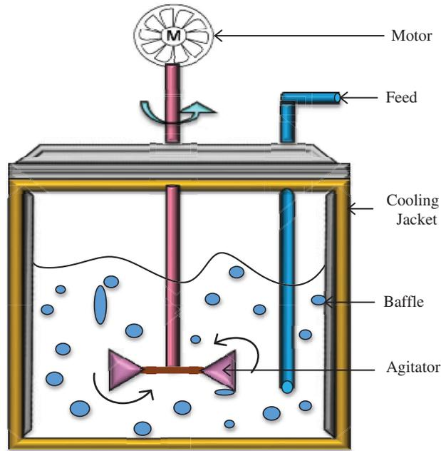
**Figure 3:** Continuous stirred-tank reactor
