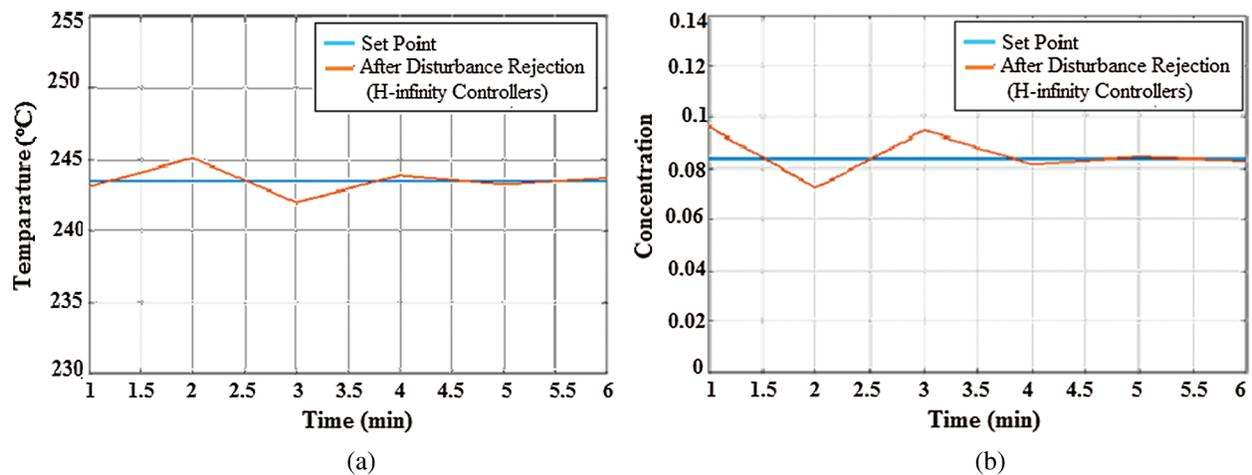
**Figure 8:** CSTR after disturbance Rejection (a) Temperature (b) Concentration
