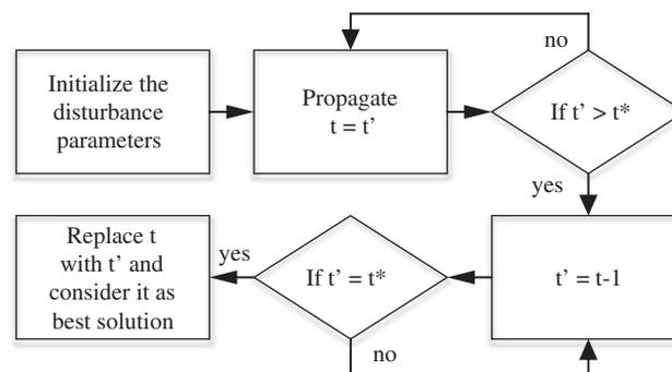
**Figure 5:** Block diagram of WWO optimization-based  $H_\infty$  controller
