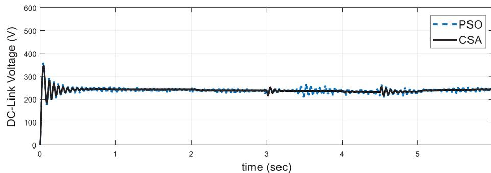
**Figure 10:** DC-Link voltage with step-change in the wind speed, the irradiation level, and the load based on PSO and CSA
