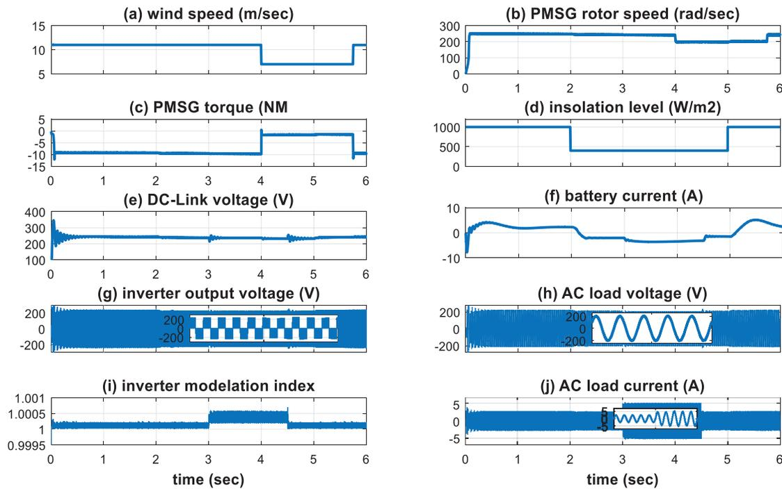
**Figure 9:** The simulation results with step-change in the wind speed, the irradiation level, and the load based on CSA with parameters change. (a) Wind speed (b) PMSG shaft speed (c) PMSG shaft torque (d) PV irradiation level (e) DC-Link voltage (f) Battery current (g) Inverter voltage (h) Load voltage (i) Inverter modulation index (j) Load current
