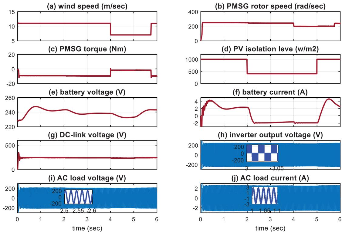
**Figure 7:** The simulation results with step-change in the wind speed and the solar irradiation based on CSA (a) Wind speed (b) PMSG shaft speed (c) PMSG shaft torque (d) PV irradiation level (e) Battery voltage (f) Battery current (g) DC-Link voltage (h) Inverter voltage (i) Load voltage (j) Load current
