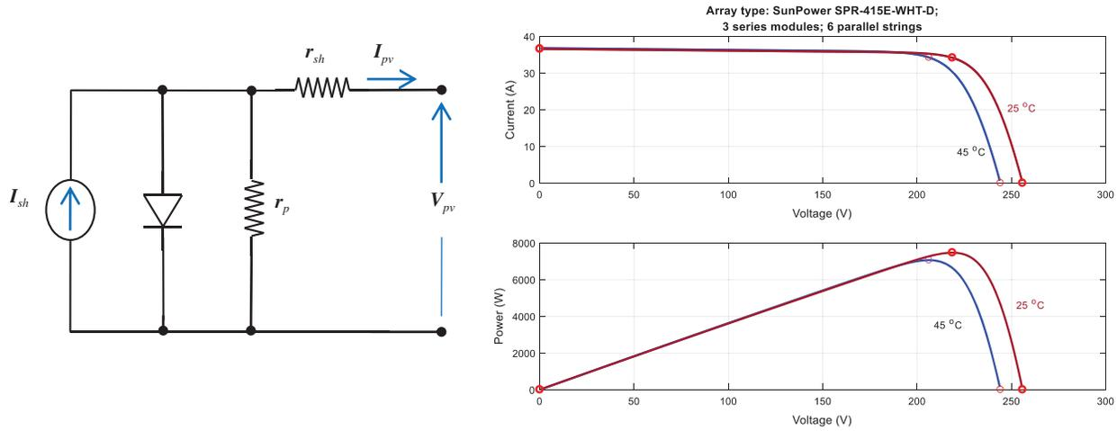
**Figure 2:** The PV array equivalent circuit model
