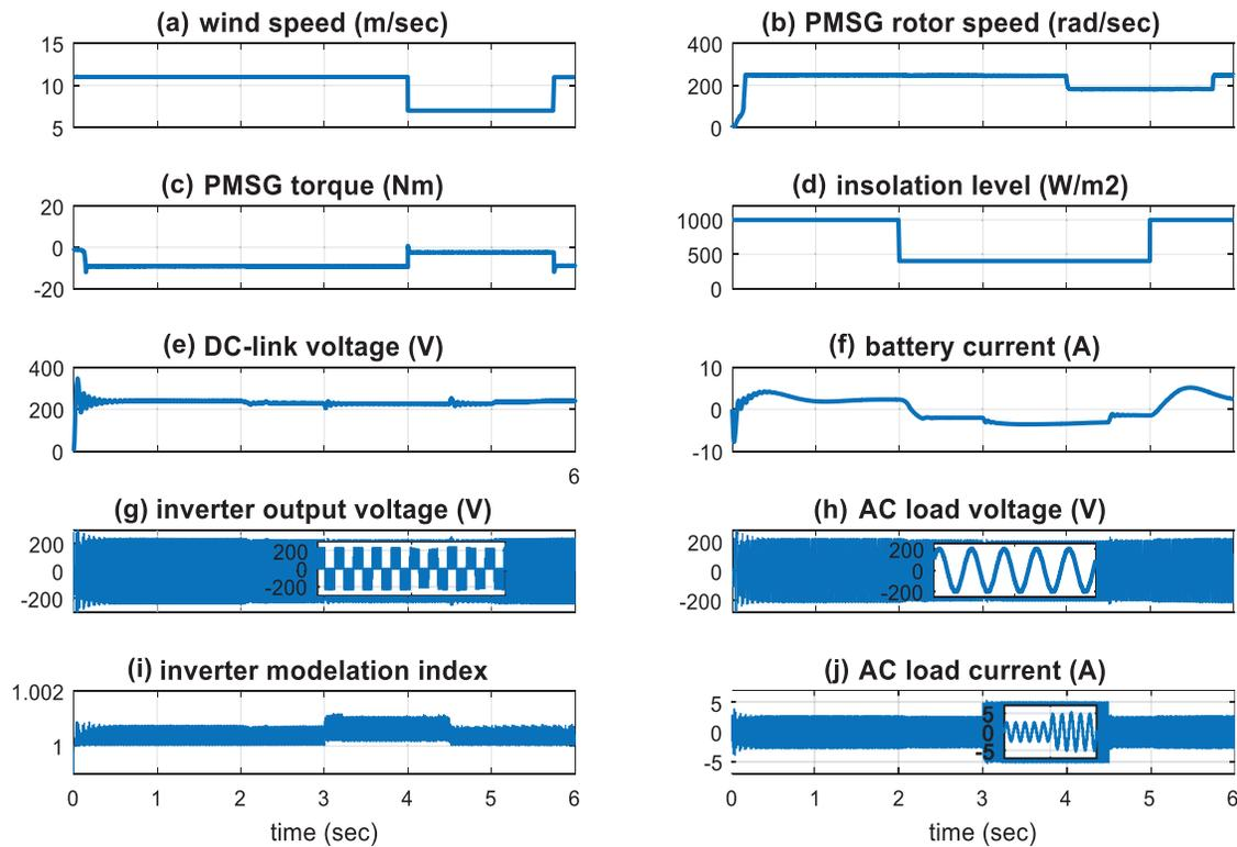
**Figure 8:** The simulation results with step-change in the wind speed, the irradiation level, and the load based on CSA (a) Wind speed (b) PMSG shaft speed (c) PMSG shaft torque (d) PV irradiation level (e) DC-Link voltage (f) Battery current (g) Inverter voltage(h) Load voltage (i) Inverter modulation index (j) Load current
