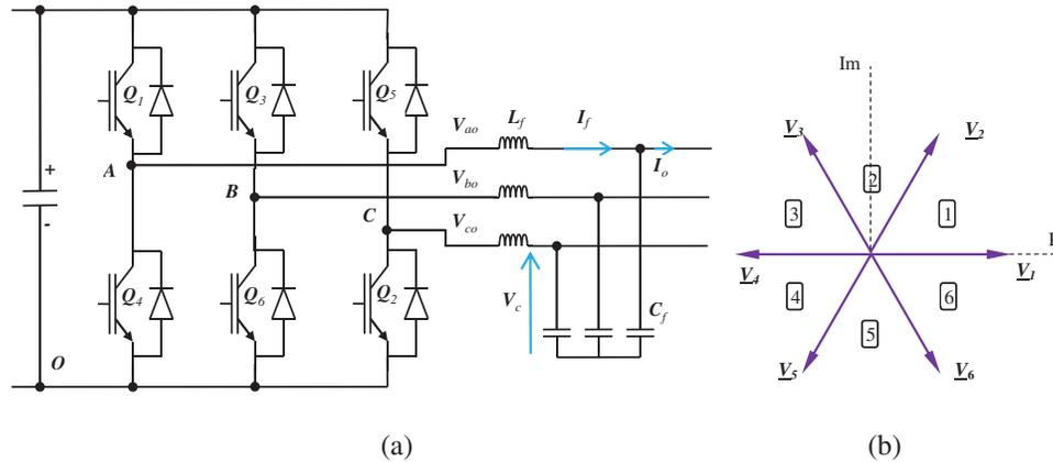
**Figure 4:** (a) The 3- $\phi$  inverter power circuit (b) The 3- $\phi$  inverter space vectors
