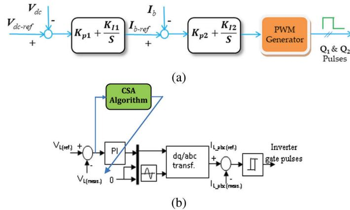
**Figure 5:** The block diagram of the (a) DC/DC controller (b) DC/AC controller
