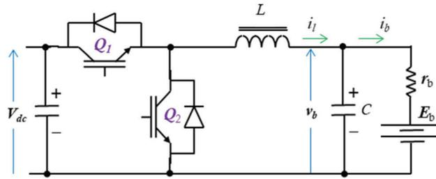
Figure 3: The DC/DC converter circuit
