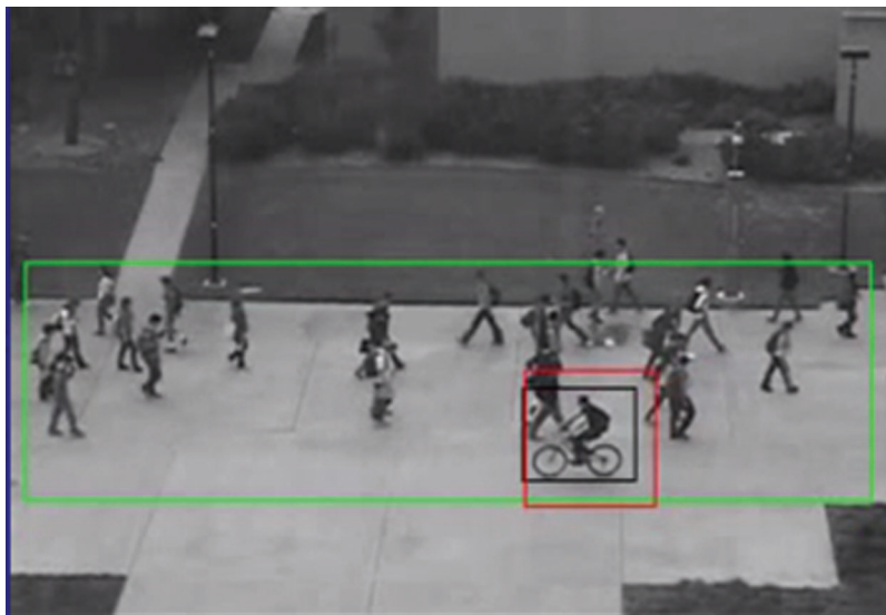
Figure 6: Human riding bicycle in pedestrian lane detected as anomaly and highlighted in red
