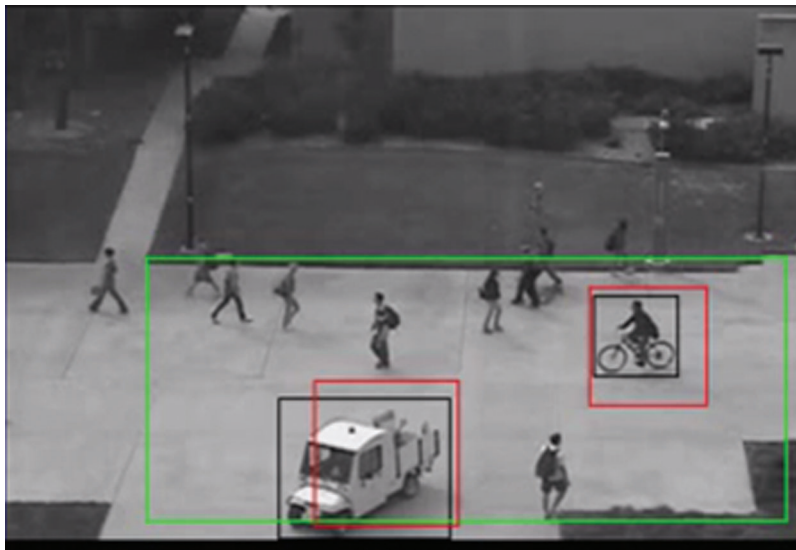
Figure 7: A bicycle and truck driven in pedestrian lane detected as anomaly and highlighted in red
