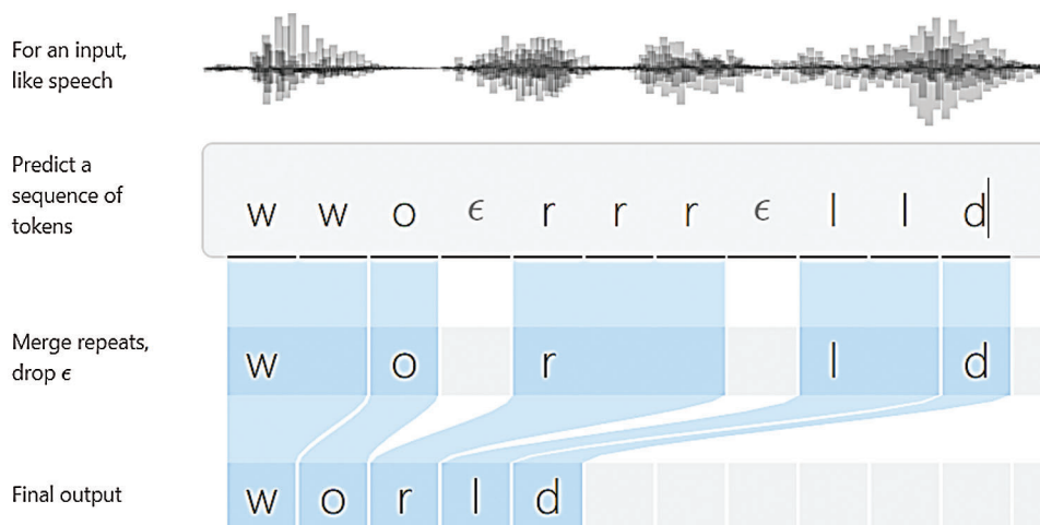
Figure 2: Working of connectionist temporal classification (CTC) [26]. CTC converts the predicted sequence of tokens to valid words with higher probability. In the predicted sequence ‘wwo rrr ll d’, the pause and the repeated tokens are dropped, giving the final output as ‘world’ with highest probability
