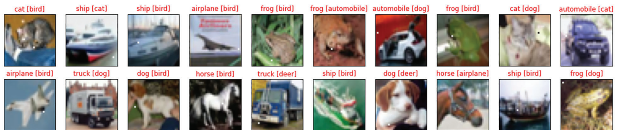
Figure 5: Adversarial example created by single pixel attack [41], one of the score-based attacks. The target model misclassifies adversarial examples; labels in red color are misclassified
