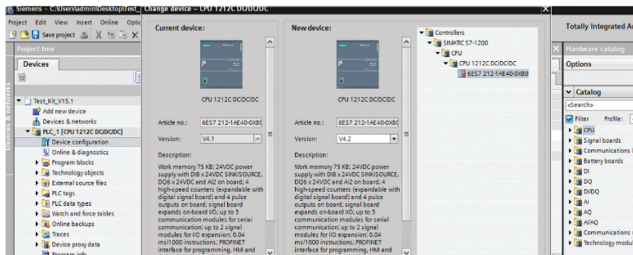
Figure 12: PLC firmware upgrade with programming tool
