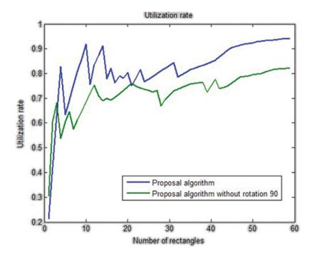
Figure 6: The utilization rate of the proposed algorithm with & without the rotation step
