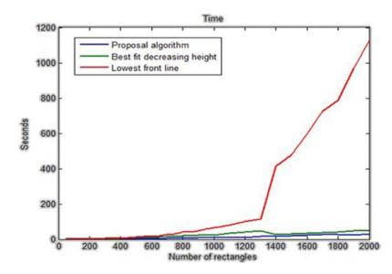
Figure 8: The running time of the Best-Fit, the front-line, and the proposed algorithms with random data
