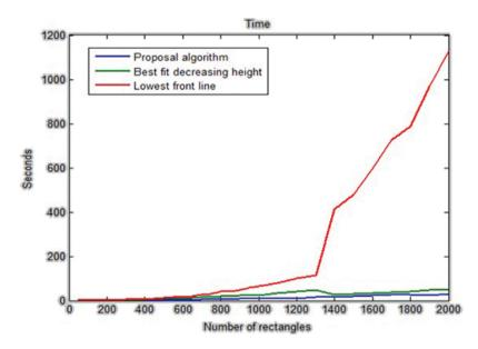
Figure 4: The running time of the Best-Fit decreasing height algorithm, the lowest front-line strategy, and the proposed algorithm
