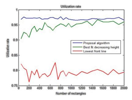
Figure 7: The utilization rate of the Best-Fit, front-line, and proposed algorithms with random data
