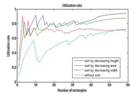
Figure 5: The utilization rate of the proposed algorithm with different sorting
