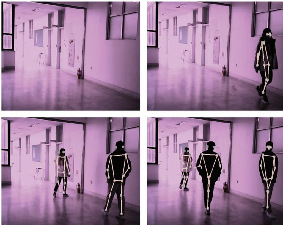
**Figure 6:** The output of the PoseNet model with MobileNet v1 for a real-time video from the C270 HD webcam installed on the AIoT edge device
