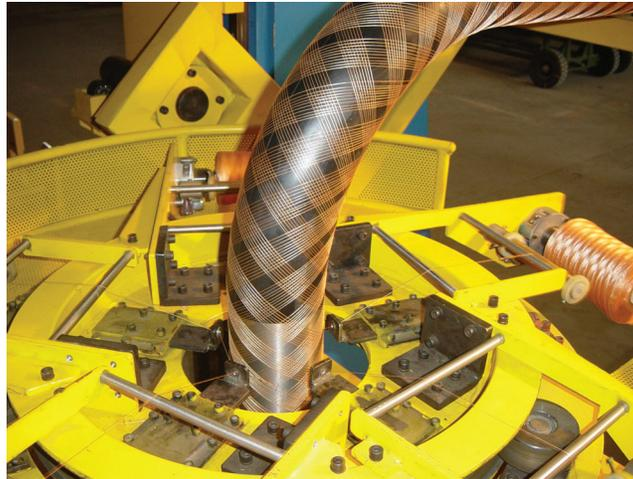
**Figure 6:** Composite elbow winding pattern used in 3-axis winding machine experiment
