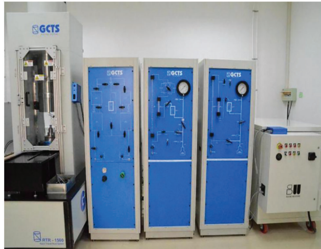
Figure 3: High-temperature rock mass triaxial testing machine
