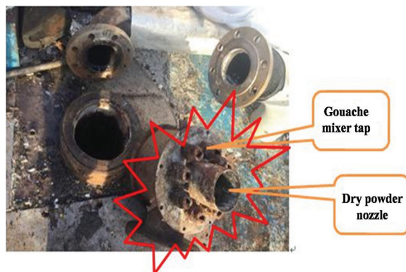
Figure 1: Schematic diagram of offshore water-powder mixer
