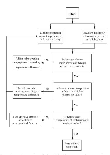
Figure 7: Designed flow chart of regulation balancing system for secondary pipeline network
