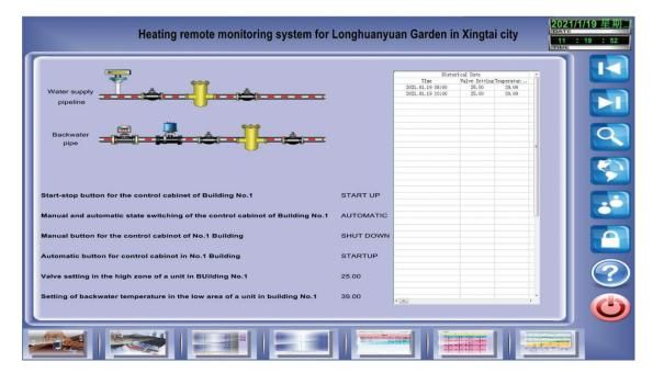
Figure 4: Remote building device control interface
