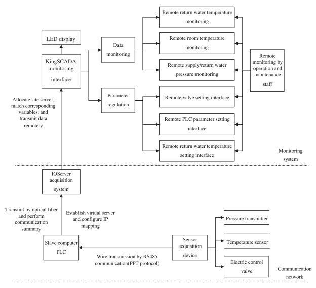
Figure 1: Remote monitoring system
