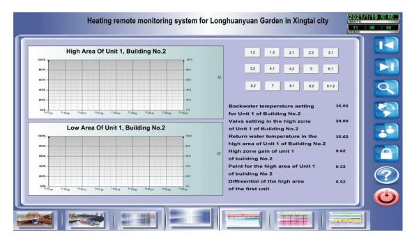
Figure 5: Remote PLC regulation interface
