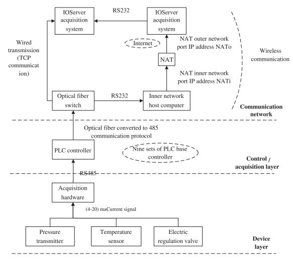
Figure 6: Remote communication flow
