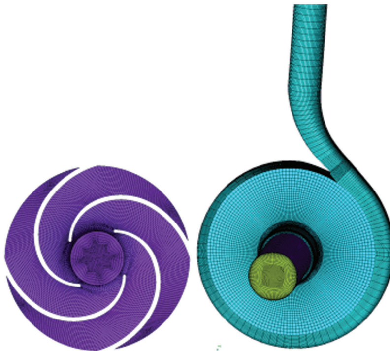
Figure 2: Impeller grid and full flow field grid assembly diagram
