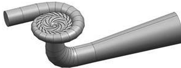
Figure 2: The basic model of a Francis turbine
