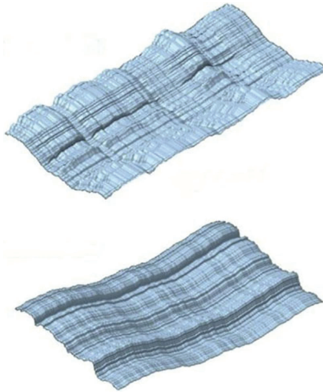
Figure 12: Typical roughness profiles for JRC = 10–12, 18–20 used by Huang et al. [74]
