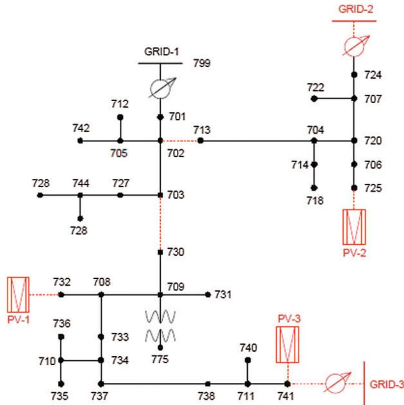
Figure 5: Modified IEEE 37-node test feeder
