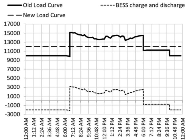
**Figure 10:** Old & new load curves, and BESS charging/discharging capacities
