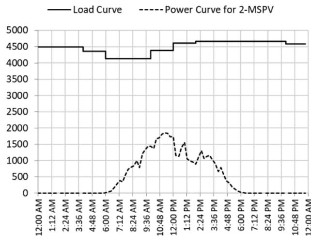
**Figure 6:** Load curve and maximum power for two MSPVs
