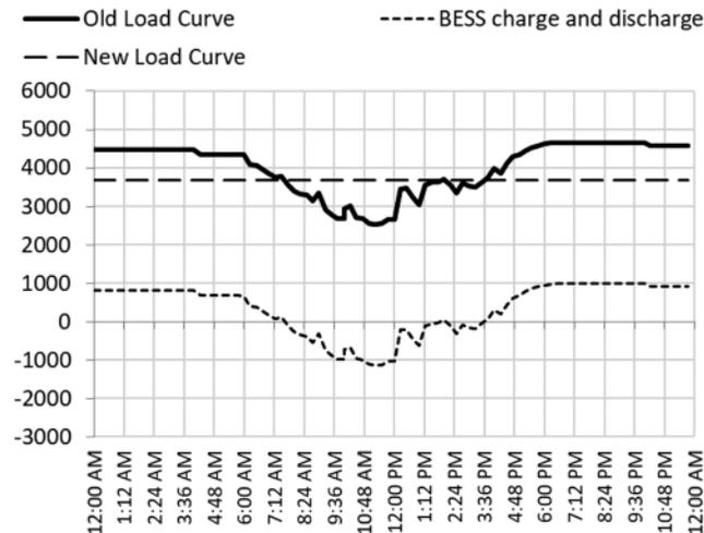
**Figure 7:** Old & new load curves, and BESS charging/discharging capacities
