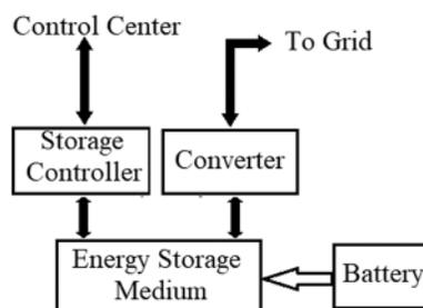
**Figure 1:** BESS diagram
