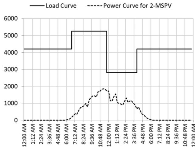
**Figure 9:** Load curve and maximum power for two MSPVs
