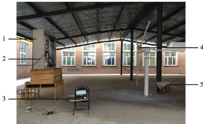
Figure 3: Icing test bench for wind power equipment. 1. Power input device fan, 2. Atomized water spray device, 3. Data collection device, 4. Wind generator, 5. Power storage box
