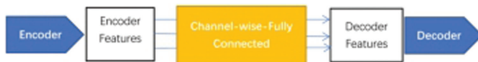
Figure 1: In the context encoder, we generally reduce the number of parameters in the network by using a channel-wise fully connected layer which employs convolution to pass information between channels
