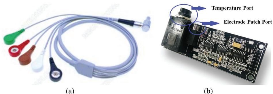
Figure 6: (a) Wire and electrode patch; (b) body temperature and respiration rate modules
