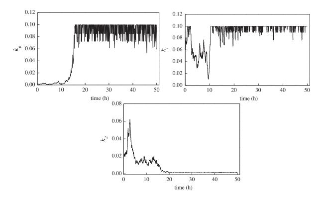
**Figure 5:** Variation of  $k_p$ ,  $k_i$  and  $k_d$  in the batch using the DE-PID control strategy
