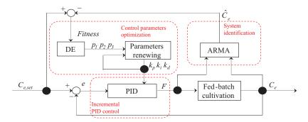
Figure 1: Schematic diagram of the DE-PID controller
