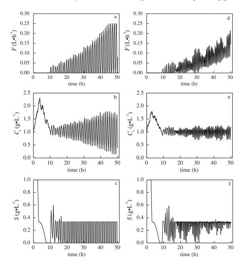
**Figure 2:** Profiles of substrate feed rate (F), ethanol concentration ( $C_e$ ) and glucose concentration (S) under PID and DE-PID control strategies. a, b and c: profiles under PID control; d, e and f: profiles under DE-PID control
