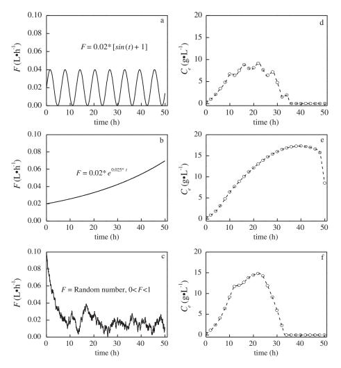
**Figure 4:** Glucose feed rate (*F*) profiles, and the corresponding real and predicted ethanol concentrations  $(C_e)$ . a, b and c: *F* profiles with sine, exponential and random curves, respectively; d, e and f: real and predicted  $C_e$  with sine, exponential and random curve feed rate profiles, respectively. Open circles: real  $C_e$ ; dash lines: predicted  $C_e$
