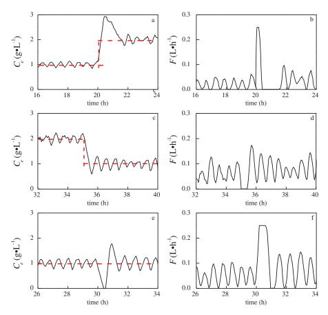
**Figure 6:** The robustness of the DE-PID controller in response to ethanol concentration set-point changes and disturbance during fermentation. a and b: changing patterns of ethanol concentration ( $C_e$ ) and glucose feed rate (F) to a  $C_e$  set-point change from 1 g•L<sup>-1</sup> to 2 g•L<sup>-1</sup>; c and d: changing patterns of  $C_e$  and F to  $C_e$  a set-point change from 2 g•L<sup>-1</sup> to 1 g•L<sup>-1</sup>; e and f: changing patterns of  $C_e$  and F to a pump fault
