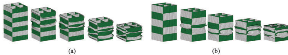
Figure 9: Deformation process of two nanocrystallization distribution types (a) 7 stripes of Type A (b) 5 stripes of Type B
