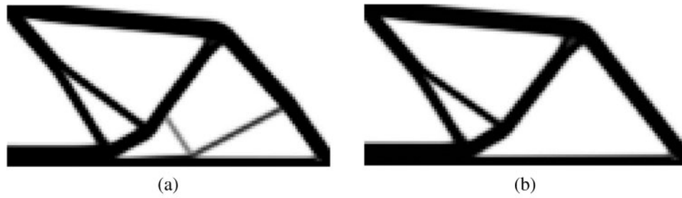
Figure 9: Comparison of FEM-TO and PGD-TO results for a half MBB beam. (a) FEM-TO (b) PGD-TO
