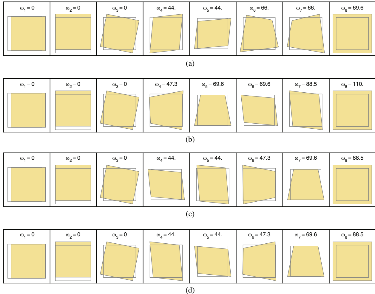
Figure 3: Eigenfrequencies \omega_n and modeshapes for single element with free-free boundary condition and stabilization parameters \beta^{stat} = \beta^{dyn} = 0.4 (a) Eigenfrequencies \omega_n and modeshapes for FEM Q1 (b) Eigenfrequencies \omega_n and modeshapes for VEM Q1 Stab (c) Eigenfrequencies \omega_n and modeshapes for VEM Q1 BI Stab (d) Eigenfrequencies \omega_n and modeshapes for VEM Q1-I Stab
