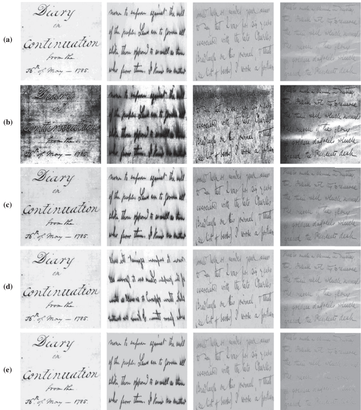
Figure 4: (a) Original image, (b) HE, (c) Butterworth Homomorphic, (d) Difference of Gaussian (DoG), (e) Proposed method
