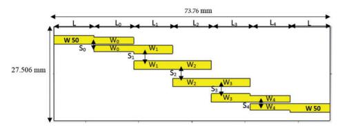
Figure 6: Parallel-coupled line layout using FR4
