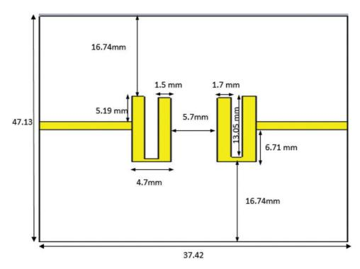
Figure 11: Physical layout on the top layer (RO3003)
