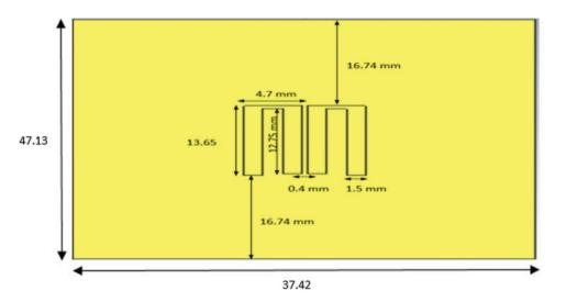
Figure 12: Physical layout on the inner layer (RO3003)
