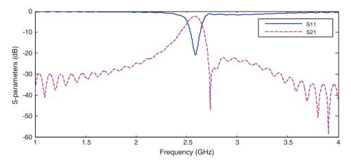
Figure 16: Simulated response of S-parameters (FR4)
