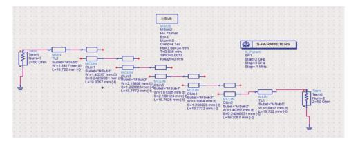
Figure 4: Parallel coupled line band-pass filter model (RO3003)
