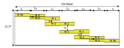
Figure 5: Parallel-coupled line layout using R03003
