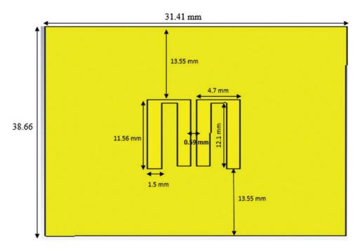
Figure 10: Physical layout on the inner layer (FR4)
