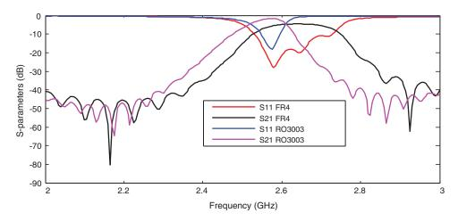
Figure 20: Comparison of simulated S-parameters PCL filter
