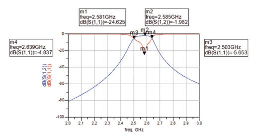
Figure 17: Simulated S-parameters of PCL filter using ADS (RO3003)
