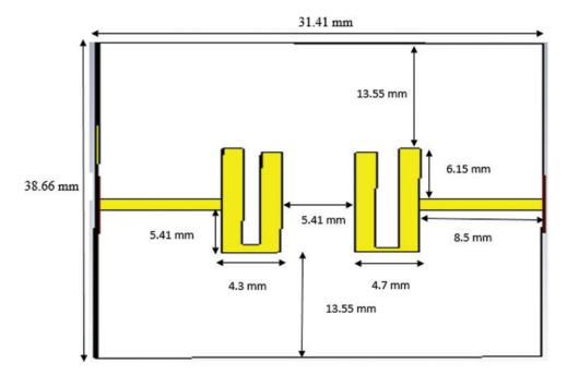
Figure 9: Physical layout on the top layer (FR4)
