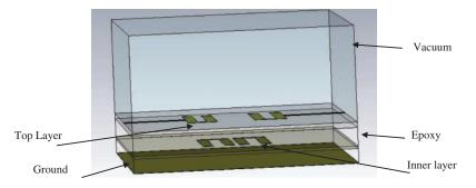
Figure 8: Construction of multilayer hairpin band-pass filter
