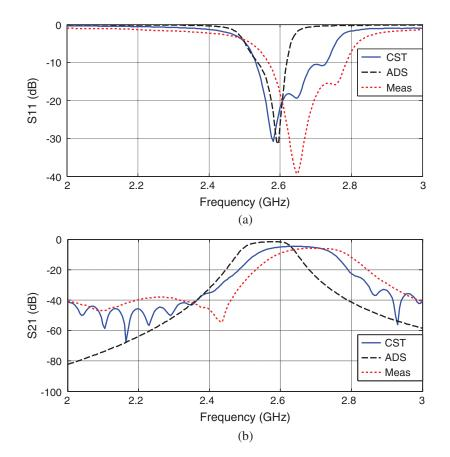
Figure 15: Comparison of measured and simulated S-parameters of the PCL filter (a) S11, (b) S21 using FR4
