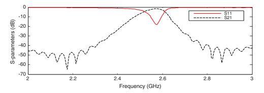
Figure 18: Simulated S-parameters of PCL filter using CST(RO3003)
