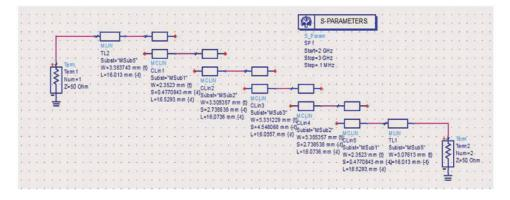
Figure 3: Parallel coupled line band-pass filter model (FR4)
