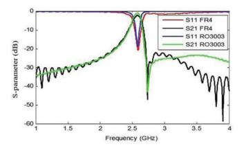
Figure 21: Comparison of simulated S-parameters ML filter
