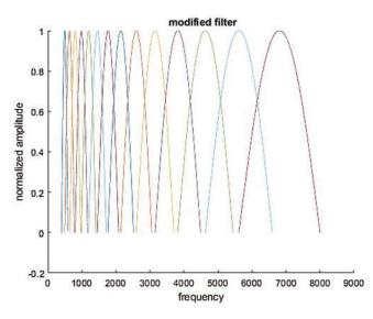
Figure 8: Sine-based filter bank
