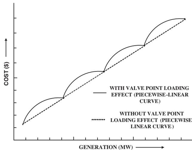
**Figure 1:** Cost characteristics of fossil fuel-based generator
