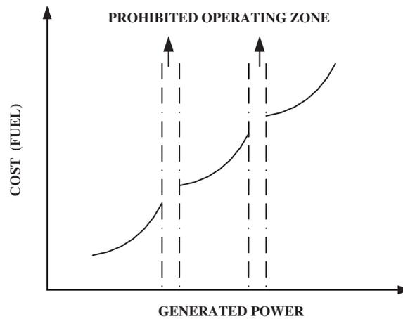
Figure 2: Generator characteristics with existing prohibited zones
