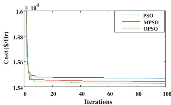
**Figure 3:** Convergence characteristics for case 1 with 1263 MW load demand
