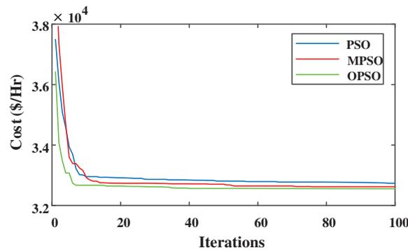
Figure 6: Convergence characteristics of case 2 for fifteen generating units
