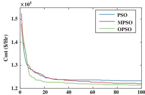
Figure 7: Convergence characteristics for test system 3 with 40 generators
