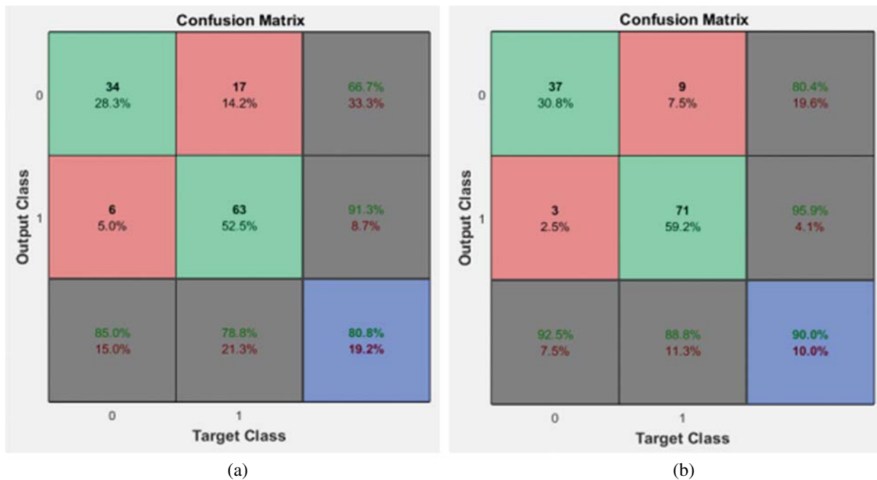
Figure 6: Confusion matrices of the 2nd stage SMC system (a) local properties (b) DRLBP
