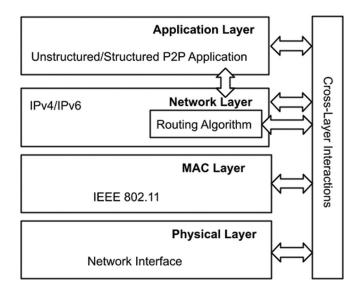
Figure 1: Proposed addressed cross-layered architecture
