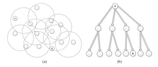
Figure 4: Searching using naive flooding technique (a) searching using broadcast by flooding technique (b) d-ary tree representation
