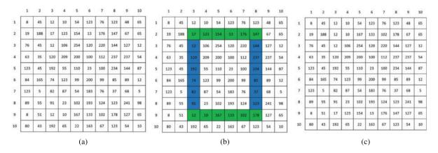
**Figure 4:** A demonstration of swapping operation on a  $10 \times 10$  sized image: (a) A  $10 \times 10$  sized image; (b) Selection of rectangle with top left corner (2, 3) and bottom right corner (9, 8); (c) Image after the swapping of horizontal lines with each other and the swapping of vertical lines with each other
