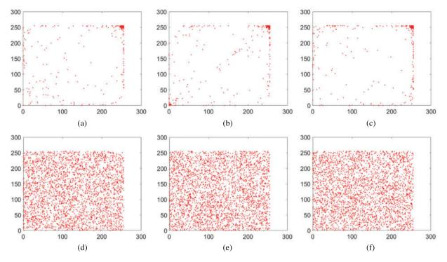
**Figure 11:** Correlation distribution for agreement 1 image (Image type, Direction): (a) (Plain, horizontal); (b) (Plain, vertical); (c) (Plain, diagonal); (d) (Cipher, horizontal); (e) (Cipher, vertical); (f) (Cipher, diagonal)
